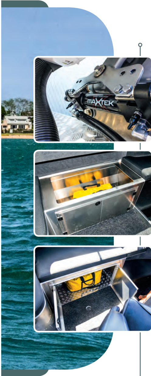
Inserts from top: Larger outboards require some muscle and a Maxtek Hydraulic steering system is fitted; Storage space under the bench seating can be reached under the squabs or through gates in the front face.
