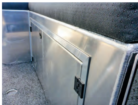
The section of seat across the rear of the cabin features a reversing bolster forming a great spot to watch lures; The welding has that smooth, flowing look reminiscent of a stack of silver coins that have been tipped over.
