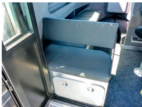
The section of seat across the rear of the cabin features a reversing bolster forming a great spot to watch lures; The welding has that smooth, flowing look reminiscent of a stack of silver coins that have been tipped over.
