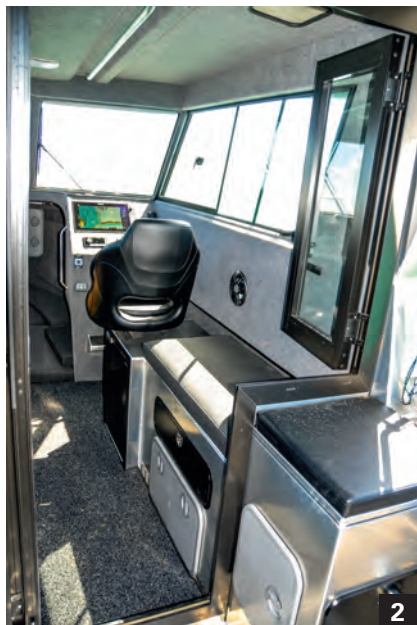
1) The port side platform cage includes a section that can fold-down to form an 'H'-type boarding ladder; 2) Lockable bi-fold cabin doors and swing window provide ventilation and communication between the helm and the cockpit; 3) The bow rail construction has a fold-down boarding ladder incorporated.
