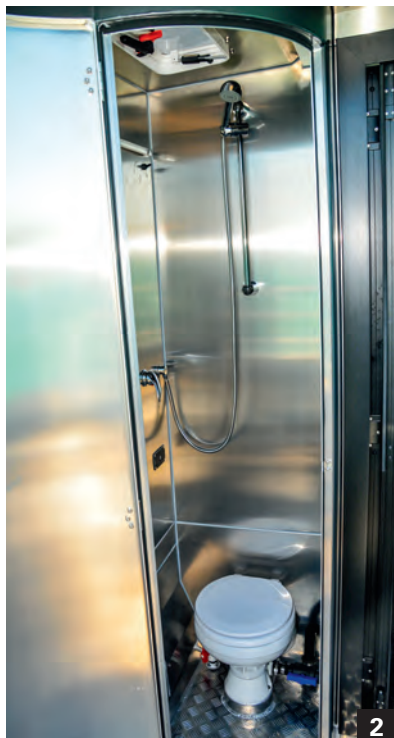
1) The Kiwi-Kraft 795 is a smooth, dry rider; 2. An enclosed flush toilet and hot-and-cold freshwater shower is fitted in the corner of the cockpit; 3) A locker set against the rear cabin bulkhead houses the gas bottle, califont, sink and bench seat; 4) Behind the helm seat is a Dometic three-burner stove with a drawer and locker beneath; 5) The helm seat is a comfortably upholstered bucket seat with roll-back bolster and footrest; 6) The forward passenger bench seat has a reversible back rest and stowage underneath.
