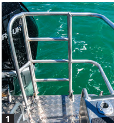
1) The port side platform cage includes a section that can fold-down to form an 'H'-type boarding ladder; 2) Lockable bi-fold cabin doors and swing window provide ventilation and communication between the helm and the cockpit; 3) The bow rail construction has a fold-down boarding ladder incorporated.
