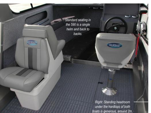
The 590 Sport has port side access with twin lockers in the centre and a starboard bait board.
