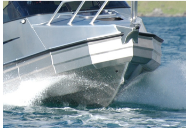
This shot shows how the bow shape turns the spray down and away from the boat.
