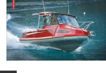
Kiwi Engineering uses its own aluminium boat technology, called Kiwi Hushtec, that incorporates a variable deadrise hull coupled to the cushioning pontoons. This, according to Rodney Harris, is to increase straightline speed and improve manoeuvrability and all-round handling in any conditions.
